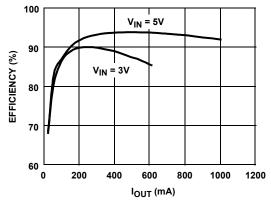
FIGURE 2. VBOOST EFFICIENCY vs IOUT (P MODE)
