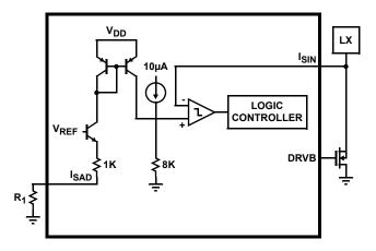
FIGURE 26. CURRENT LIMIT BLOCK DIAGRAM
