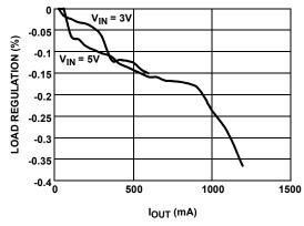
FIGURE 4. VBOOST LOAD REGULATION (PI MODE)
