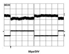
FIGURE 21. VLOGIC TRANSIENT RESPONSE
