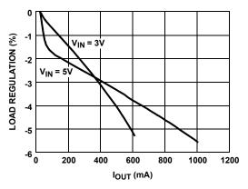
FIGURE 5. VBOOST LOAD REGULATION (P MODE)
