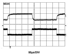
FIGURE 22. V<sub>ON</sub> TRANSIENT RESPONSE
