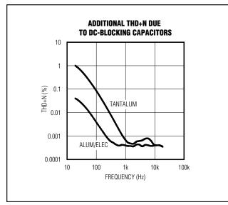
Figure 4. Distortion Contributed by DC-Blocking Capacitors
