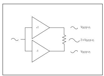
Figure 9. Bridge-Tied Load Configuration
