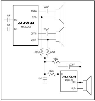
Figure 11. Stereo Plus Subwoofer Application Circuit
