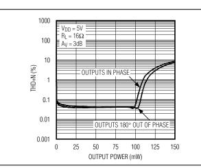
Figure 10. Total Harmonic Distortion Plus Noise vs. Output Power with Inputs In/Out of Phase (Headphone Mode)
