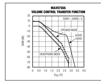
Figure 7a. Volume Control Transfer Function
