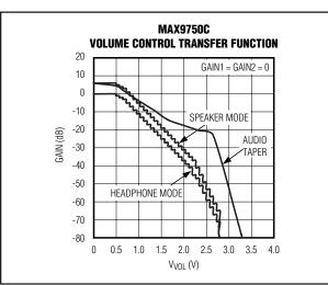
Figure 7c. Volume Control Transfer Function
