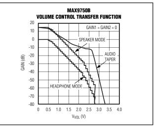
Figure 7b. Volume Control Transfer Function
