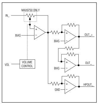
Figure 1. MAX9750/MAX9751 Signal Path
