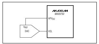
Figure 6. Volume Control Circuit
