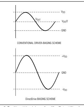
Figure 2. Traditional Headphone Amplifier Output Waveform vs. DirectDrive Headphone Amplifier Output Waveform
