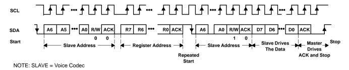
Figure 8. I<sup>2</sup>C Read From Voice Codec: Protocol A
