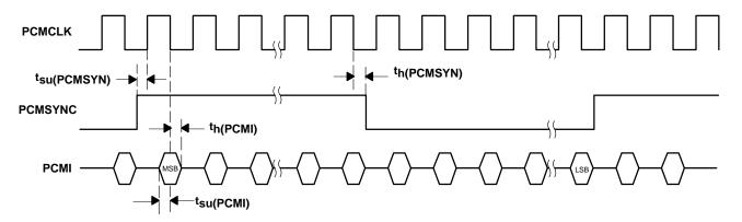
Figure 4. Receive Timing Diagram, 128 kHz
