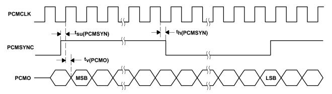
Figure 5. Transmit Timing Diagram, 128 kHz
