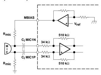
Figure 12. Typical Microphone Interface
