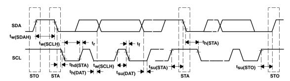
Figure 3. I<sup>2</sup>C-Bus Timing Diagram
