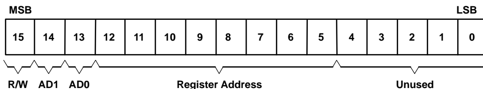
Figure 5. Bit Assignment and Definition for Slot-0 Word
