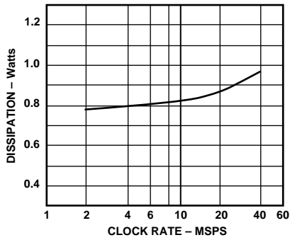
Figure 11. Power Dissipation vs. Clock Rate
