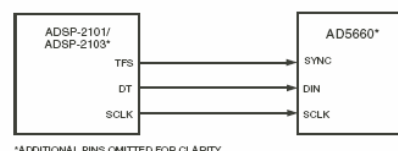
Figure 26. AD5660 to ADSP-2101/ADSP-2103 Interface
