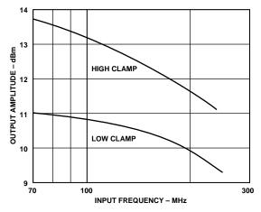
Figure 5. Clamp Level vs. Frequency
