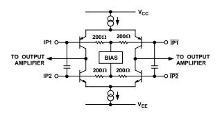
Figure 13. Equivalent Input Circuit
