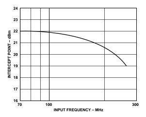
Figure 2. 3rd Order Intercept (IP3) vs. Frequency
