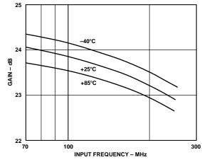
Figure 3. Gain vs. Frequency
