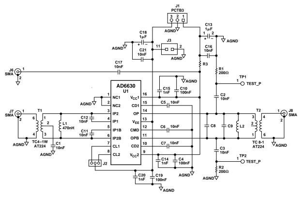
Figure 14. Evaluation Board Schematic
