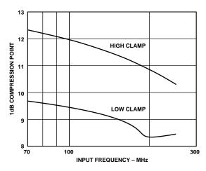
Figure 4. 1 dB Compression Point (Typical)
