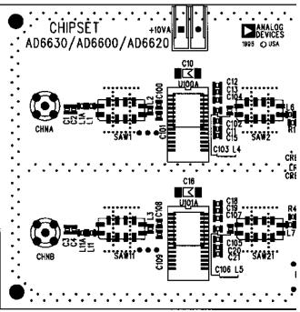
Figure 12. Reference Design Component Placement (Two Channels Shown)
