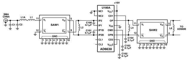
Figure 9. Reference Design Schematic (One Channel)
