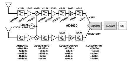
Figure 6. GSM Design Example
