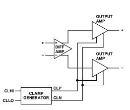
Figure 11. Functional Block Diagram
