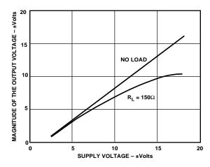
Figure 2. Output Voltage Swing vs. Supply
