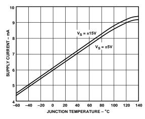
Figure 4. Supply Current vs. Junction Temperature
