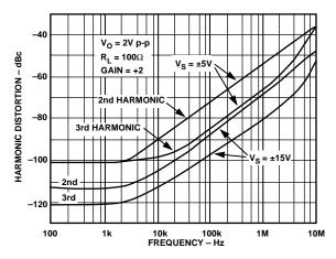
Figure 15. Harmonic Distortion vs. Frequency ( $R_L = 100 \Omega$ )
