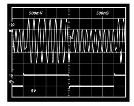
Figure 52. Channel Switching Time for the 2:1 Mux
