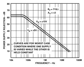
Figure 14. Power Supply Rejection vs. Frequency
