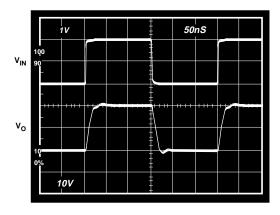
Figure 26. Large Signal Pulse Response, Gain = +10,  $R_F = 442 \,\Omega$ ,  $R_L = 400 \,\Omega$ ,  $V_S = \pm 15 \,V$
