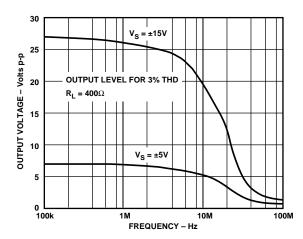
Figure 11. Large Signal Frequency Response
