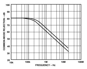
Figure 13. Common-Mode Rejection vs. Frequency
