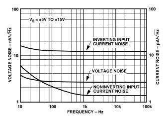
Figure 12. Input Voltage and Current Noise vs. Frequency
