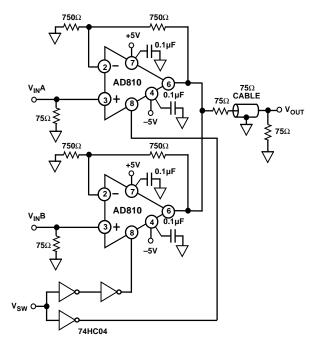
Figure 54. A Fast Switching 2:1 Video Mux
