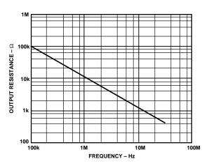
Figure 10. Output Resistance vs. Frequency, Disabled State
