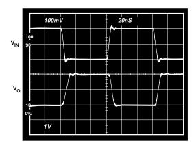
Figure 37. Small Signal Pulse Response, Gain = –10,  $R_F = 442 \, \Omega$ ,  $R_L = 150 \, \Omega$ ,  $V_S = \pm 15 \, V$
