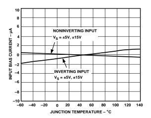
Figure 5. Input Bias Current vs. Temperature
