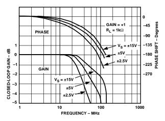
Figure 22. Closed-Loop Gain and Phase vs. Frequency, G=+1,  $R_F=1$  k $\Omega$  for  $\pm 15$  V, 910  $\Omega$  for  $\pm 5$  V and  $\pm 2.5$  V
