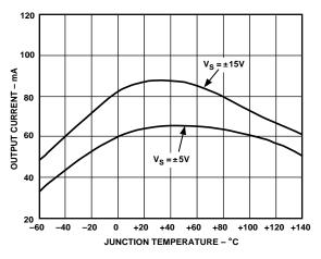
Figure 8. Linear Output Current vs. Temperature
