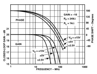
Figure 40. Closed-Loop Gain and Phase vs. Frequency, G = -10,  $R_L = 1 \text{ k}\Omega$
