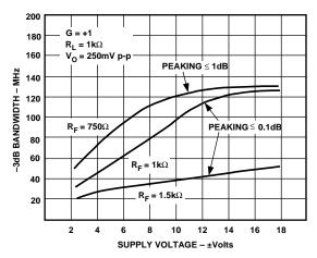
Figure 24. –3 dB Bandwidth vs. Supply Voltage G=+1,  $R_L=1~\mathrm{k}\Omega$
