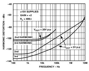
Figure 16. Harmonic Distortion vs. Frequency ( $R_L = 400 \Omega$ )
