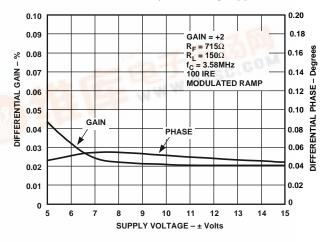
Differential Gain and Phase vs. Supply Voltage
