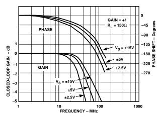
Figure 21. Closed-Loop Gain and Phase vs. Frequency, G=+1.  $R_F=1$  k $\Omega$  for  $\pm 15$  V, 910  $\Omega$  for  $\pm 5$  V and  $\pm 2.5$  V
