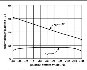
Figure 7. Short Circuit Current vs. Temperature
