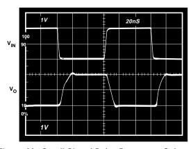
Figure 32. Small Signal Pulse Response, Gain = -1,  $R_F = 681 \,\Omega$ ,  $R_L = 150 \,\Omega$ ,  $V_S = \pm 5 \,V$
