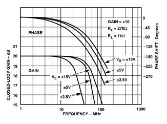
Figure 28. Closed-Loop Gain and Phase vs. Frequency, G = +10,  $R_L = 1 \text{ k}\Omega$
