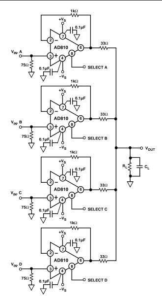
Figure 58. A 4:1 Multiplexer Driving a High Impedance
