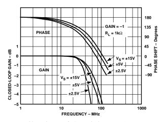
Figure 34. Closed-Loop Gain and Phase vs. Frequency, G=-1,  $R_L=1$  k $\Omega$ ,  $R_F=681$   $\Omega$  for  $V_S=\pm15$  V, 620  $\Omega$  for  $\pm5$  V and  $\pm2.5$  V
