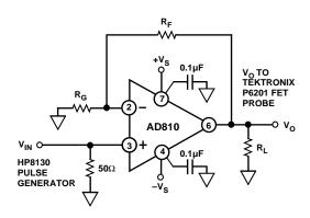
Figure 19. Noninverting Amplifier Connection
