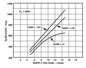
Figure 18. Slew Rate vs. Supply Voltage
