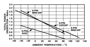
Maximum Power Dissipation vs. Temperature
