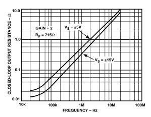
Figure 9. Closed-Loop Output Resistance vs. Frequency
