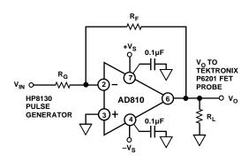
Figure 31. Inverting Amplifier Connection
