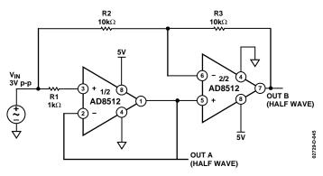
Figure 50. Half-Wave and Full-Wave Rectifier
