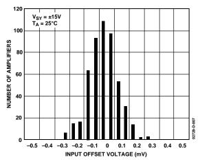
Figure 7. Input Offset Voltage Distribution
