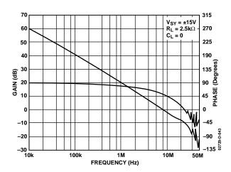
Figure 48. Frequency Response of the AD8510/AD8512/AD8513
