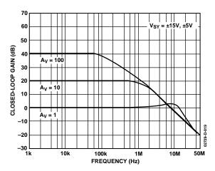
Figure 19. Closed-Loop Gain vs. Frequency
