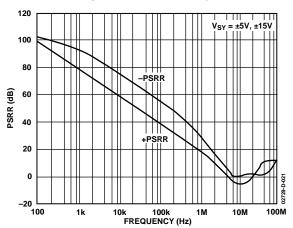
Figure 21. PSRR vs. Frequency
