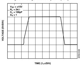
Figure 26. Large Signal Transient Response
