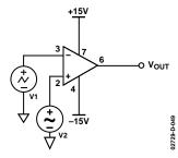
Figure 54. Pulse-Width Modulator
