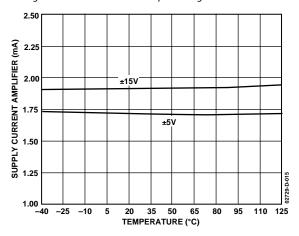
Figure 15. AD8512 Supply Current per Amplifier vs. Temperature
