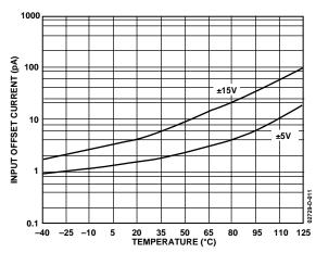
Figure 11. Input Offset Current vs. Temperature
