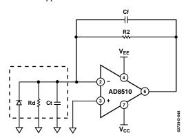
Figure 53. Equivalent Preamplifier Photodiode Circuit
