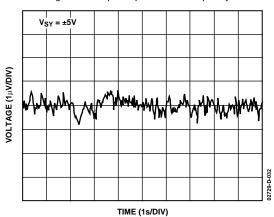
Figure 32. 0.1 Hz to 10 Hz Input Voltage Noise
