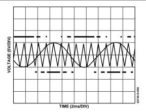
Figure 56. Pulse-Width Modulation
