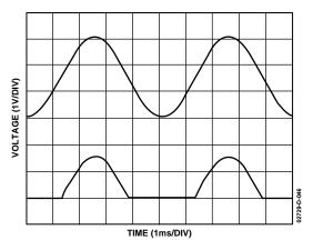
Figure 51. Half-Wave Rectifier Signal (Out A)
