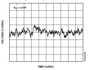
Figure 24. 0.1 Hz to 10 Hz Input Voltage Noise
