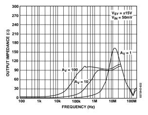
Figure 22. Output Impedance vs. Frequency
