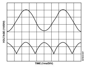
Figure 52. Full-Wave Rectifier Signal (Out B)
