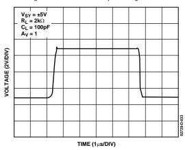
Figure 33. Large Signal Transient Response
