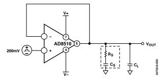
Figure 45. Snubber Network Configuration
