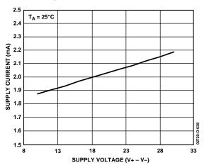
Figure 38. AD8513 Supply Current vs. Supply Voltage
