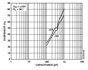
Figure 28. Small Signal Overshoot vs. Load Capacitance
