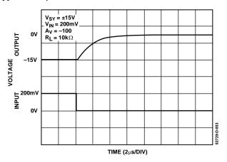
Figure 43. Positive Overload Recovery
