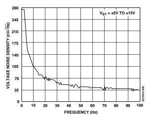
Figure 25. Voltage Noise Density vs. Frequency
