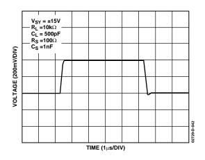
Figure 47. Capacitive Load with Snubber Network
