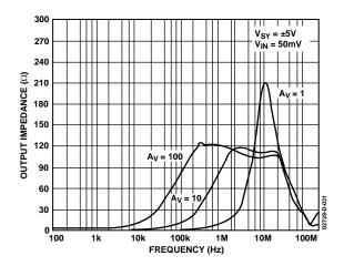
Figure 31. Output Impedance vs. Frequency
