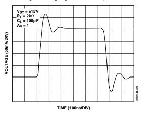
Figure 27. Small Signal Transient Response
