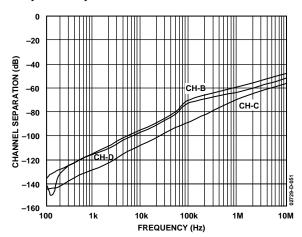
Figure 57. Channel Separation
