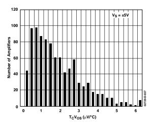
Figure 37. AD8513 T<sub>C</sub>V<sub>OS</sub> Distribution
