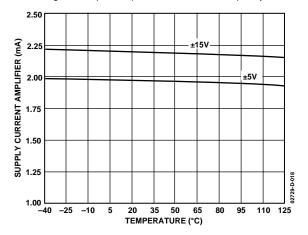
Figure 18. AD8510 Supply Current vs. Temperature
