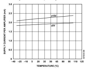
Figure 40. AD8513 Supply Current vs. Temperature
