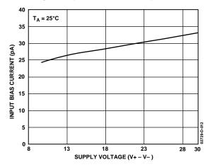
Figure 12. Input Bias Current vs. Supply Voltage
