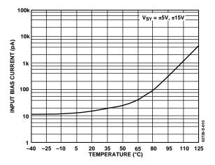
Figure 10. Input Bias Current vs. Temperature
