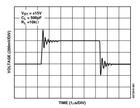
Figure 46. Capacitive Load Drive without Snubber
