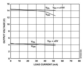
Figure 39. AD8513 Output Voltage vs. Load Current
