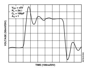
Figure 34. Small Signal Transient Response
