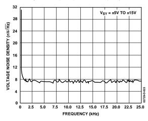
Figure 23. Voltage Noise Density
