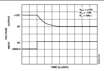
Figure 44. Negative Overload Recovery
