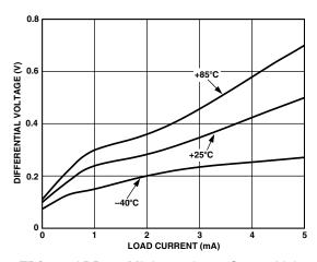
TPC 12. ADR381 Minimum Input/Output Voltage Differential vs. Load Current
