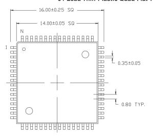
DIMENSIONS IN MILLIMETERS LEAD COPLANARITY 0.100 MAX.
