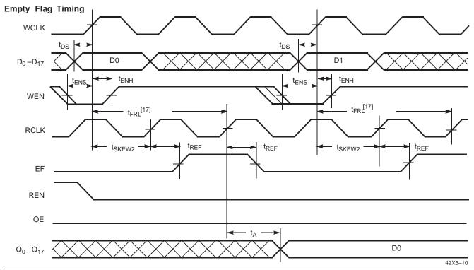
When  $t_{SKEW2} \ge$  minimum specification,  $t_{FRL}$  (maximum) =  $t_{CLK} + t_{SKEW2}$ . When  $t_{SKEW2} <$  minimum specification,  $t_{FRL}$  (maximum) = either  $2^*t_{CLK} + t_{SKEW2}$  or  $t_{CLK} + t_{SKEW2}$ . The Latency Timing applies only at the Empty Boundary (EF = LOW). The first word is available the cycle after EF goes HIGH, always.
