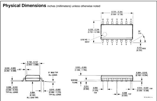
14-Lead Small Outline Integrated Circuit (SOIC), JEDEC MS-012, 0.150 Narrow Package Number M14A
