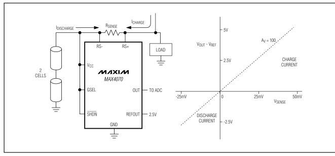
Figure 2. Bidirectional Current Monitor
