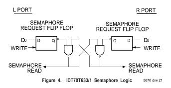
opposite side flag will now stay LOW until its semaphore request latch is written to a one. From this it is easy to understand that, if a semaphore is requested and the processor which requested it no longer needs the resource, the entire system can hang up until a one is written into that semaphore request latch.
