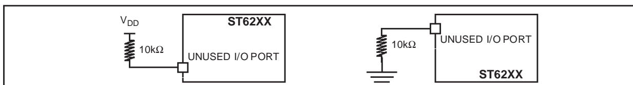
Figure 62. Two typical Applications with unused I/O Pin
