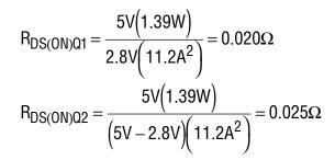
Note that while the required  $R_{DS(ON)}$  values suggest large MOSFETs, the power dissipation numbers are only 1.39W per device or less—large TO-220 packages and heat sinks are not necessarily required in high efficiency applications. Siliconix Si4410DY or International Rectifier
