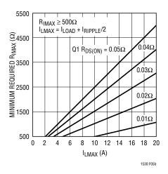
Figure 5b. Minimum Required  $R_{IMAX}$  vs  $I_{LMAX}$
