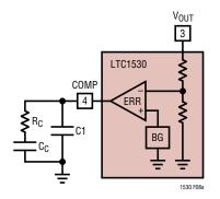
Figure 8a. Compensation Pin Hook-Up
