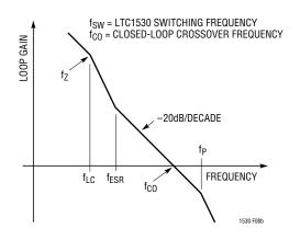
Figure 8b. Bode Plot of the LTC1530 Overall Transfer Function
