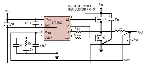
Figure 9. LTC1530 Layout Diagram
