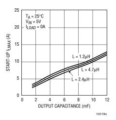
Figure 6a. Start-Up ILMAX vs Output Capacitance
