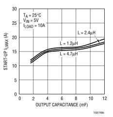
Figure 6b. Start-Up I<sub>LMAX</sub> vs Output Capacitance
