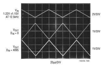
Internal Reference, REFLO/REFHI Pins, Gain Adjust and Wide Supply Voltage Range Allow 4-Quadrant Mulitplying on a 5V Single Supply
