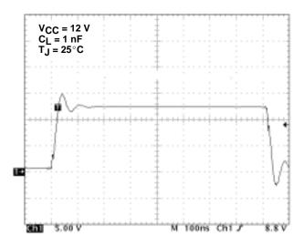
Figure 20. PWMB Rise and Fall Times
