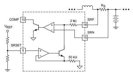
Figure 7. Battery Charge Current Input Threshold Function
