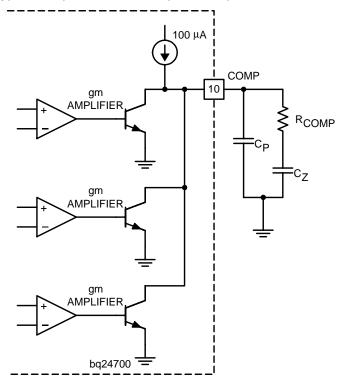
Figure 8. Type II Compensation Network
