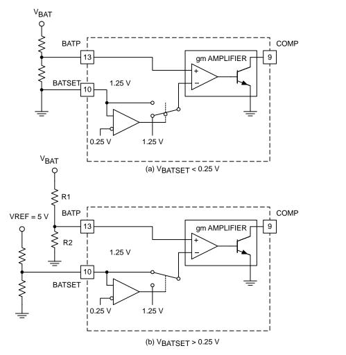
Figure 6. Battery Error Amplifier Input Multiplexing Scheme
