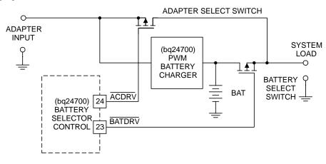
**Figure 9. Selector Control Switches**
