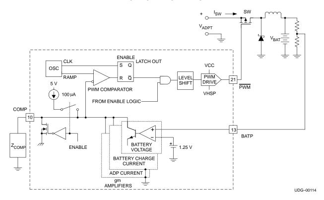
Figure 3. PWM Controller Block Diagram
