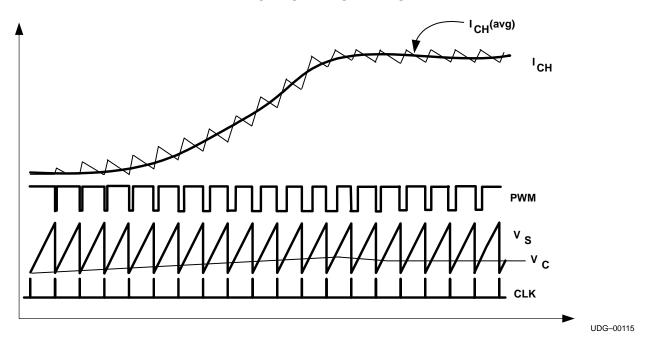
Figure 5. Typical PWM Waveforms in a Buck Converter (Including Startup)
