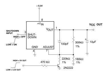
PIN 3 LOW= ENABLE OUTPUT. Q1 ON = 3.3V, Q1 OFF = 5.0V.
