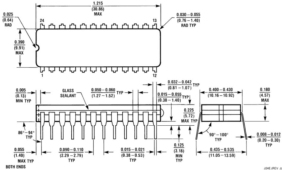
**24-Lead Ceramic Dual-In-Line Package (0.400" Wide) (D)**
