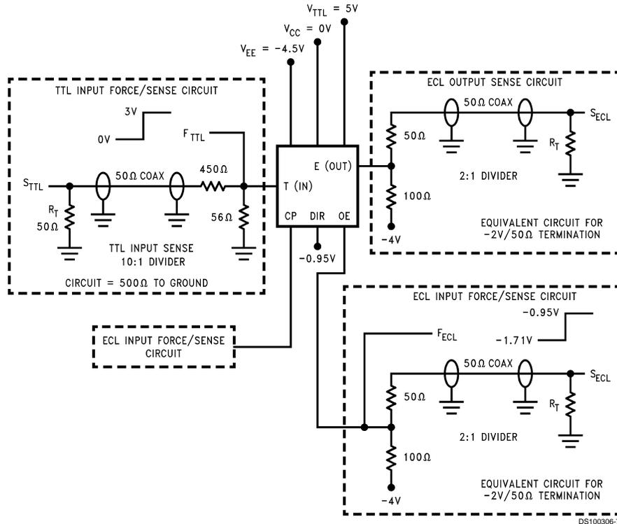
**Note 15:**  $R_T = 50\Omega$  termination resistive load. When an input or output is being monitored by a scope,  $R_T$  is supplied by the scope's  $50\Omega$  input resistance. When an input or output is not being monitored, an external  $50\Omega$  resistance must be applied to serve as  $R_T$ .
