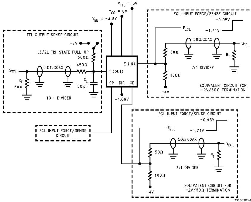
**Note 18:**  $R_T = 50\Omega$  termination resistive load. When an input or output is being monitored by a scope,  $R_T$  is supplied by the scope's  $50\Omega$  input resistance. When an input or output is not being monitored, an external  $50\Omega$  resistance must be applied to serve as  $R_T$ .
