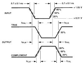
FIGURE 2. Propagation Delay and Transition Times
