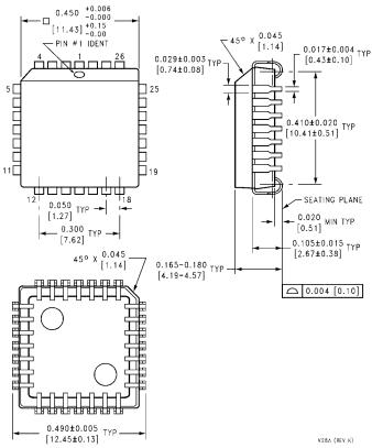
28-Lead Plastic Lead Chip Carrier (PLCC), JEDEC MO-047, 0.450 Square Package Number V28A
