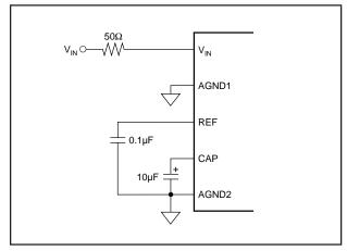
FIGURE 4b. Circuit Diagram Without External Hardware Trim.
