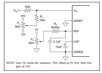
FIGURE 4a. Circuit Diagram With External Hardware Trim.
