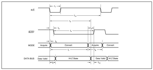
FIGURE 2. Conversion Timing with Outputs Enabled After Conversion (CS Tied Low).
