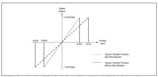
FIGURE 5. Comparison of the ADS7810 Transfer Function With and Without the  $50\Omega$  Series Resistor on  $V_{\rm IN}$
