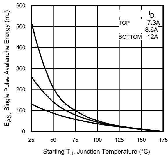
Fig 13c. Maximum Avalanche Energy vs. Drain Current
