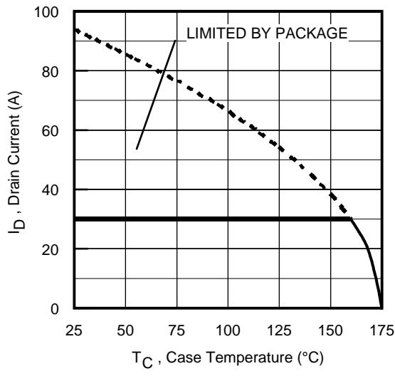
**Fig 9.** Maximum Drain Current vs.
