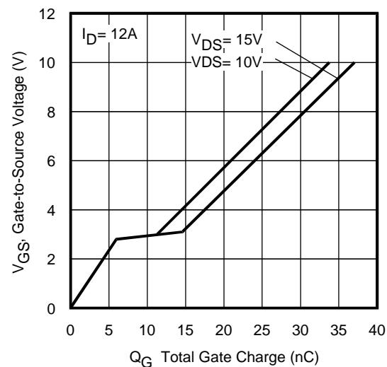
**Fig 6.** Typical Gate Charge vs.
