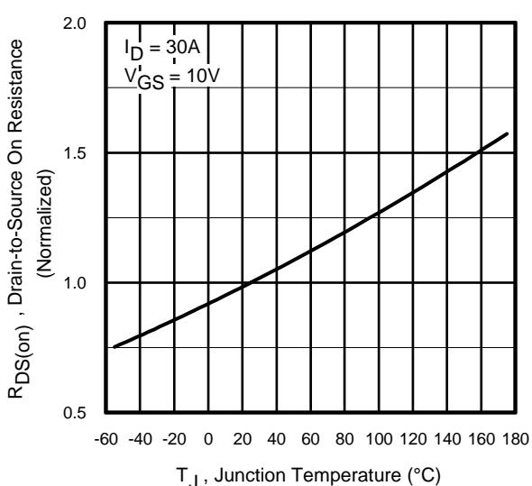
**Fig 4.** Normalized On-Resistance
