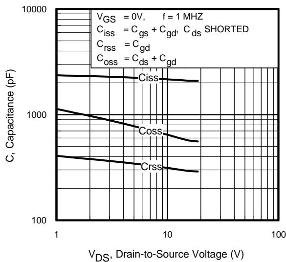
**Fig 5.** Typical Capacitance vs.
