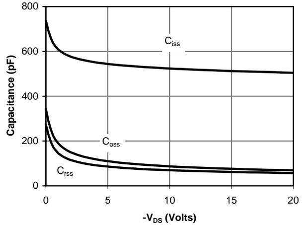
Figure 8: Capacitance Characteristics
