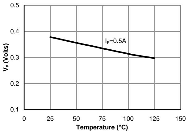
Figure 14: Schottky Forward Drop vs. Junction Temperature
