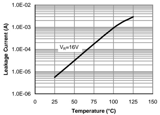
Figure 15: Schottky Leakage current vs. Junction Temperature
