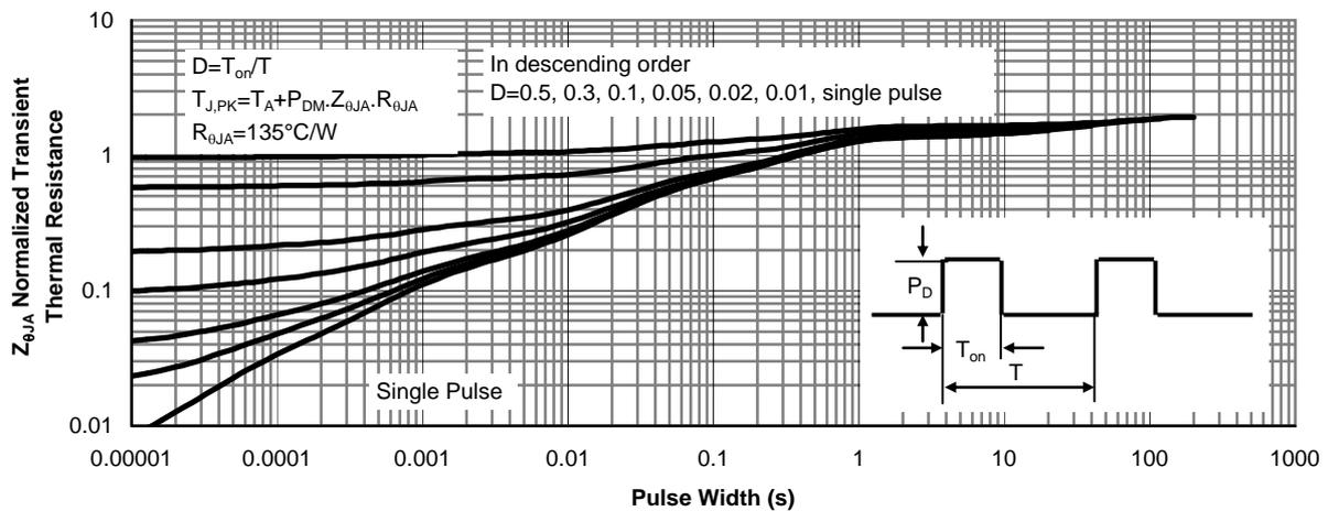
Figure 15: Schottky Normalized Maximum Transient Thermal Impedance
