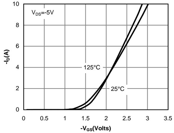
Figure 2: Transfer Characteristics
