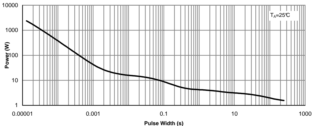
Figure 11: Single Pulse Power Rating Junction-to-Ambient (Note F)
