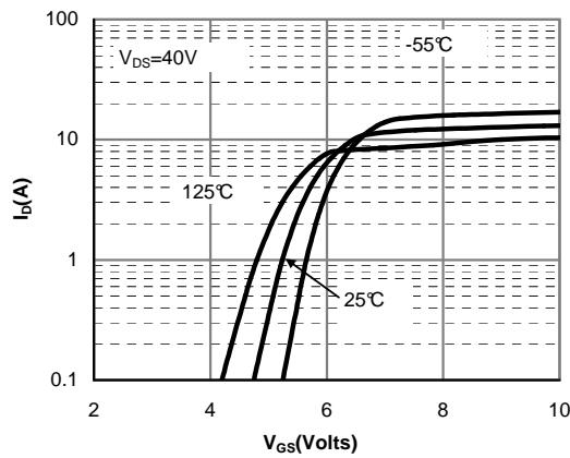
Figure 2: Transfer Characteristics
