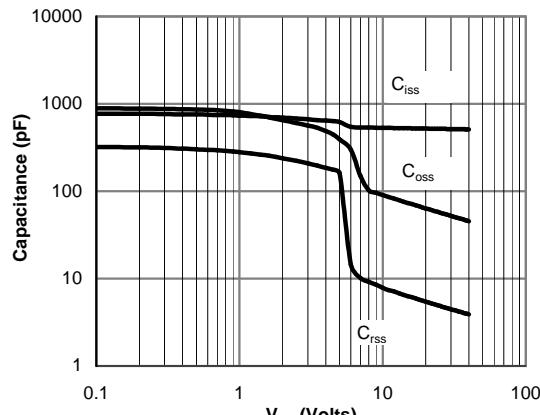
Figure 8: Capacitance Characteristics
