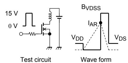
$$R_G = 25 \Omega \quad V_{DD} = 90 \text{ V}, L = 9.72 \text{ mH} \quad E_{AS} = \frac{1}{2} \cdot L \cdot I^2 \cdot \left( \frac{BVDSS}{BVDSS - V_{DD}} \right)$$
