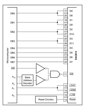
FIGURE 8. Right-Justified Data Bus Interface.
