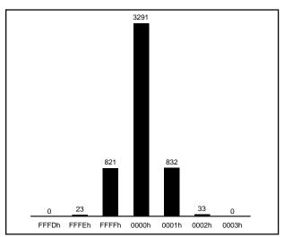
FIGURE 14. Histogram of 5,000 Conversions with Input Grounded.
