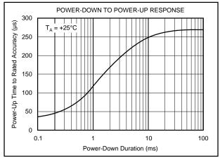
FIGURE 11. Power-Down to Power-Up Response.
