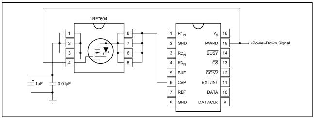
FIGURE 12. Improved Power-Up Response Circuit.
