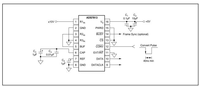
FIGURE 1a. Basic Operation, ±10V Input Range, Internal DATACLK.
