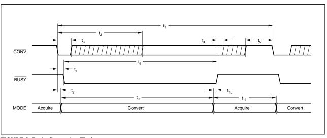
FIGURE 2. Basic Conversion Timing.
