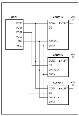
FIGURE 16. QSPI Interface to Three ADS7813s.
