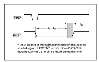
FIGURE 4. Timing of the Shift Register Update.
