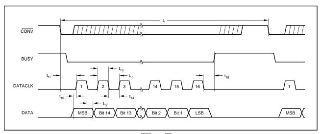
FIGURE 5. Serial Data Timing, Internal Clock (EXT/INT and CS LOW).
