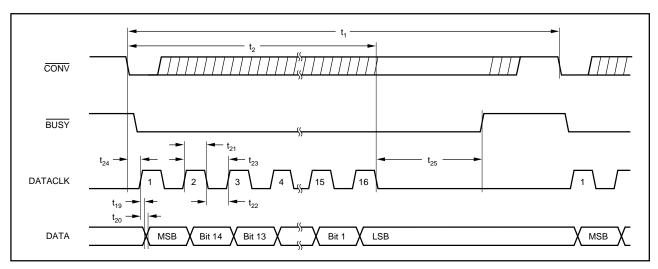
FIGURE 7. Serial Data Timing, External Clock, Clocking During the Next Conversion (EXT/INT HIGH, CS LOW).
