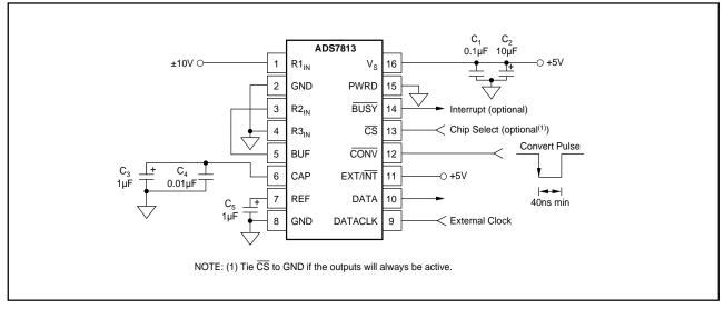
FIGURE 1b. Basic Operation, ±10V Input Range, External DATACLK.
