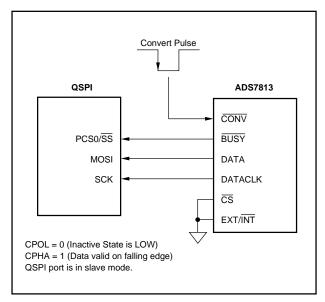
FIGURE 15. QSPI Interface to the ADS7813.
