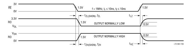
Figure 8. Receiver Enable and Disable Times
