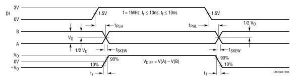
Figure 5. Driver Propagation Delays
