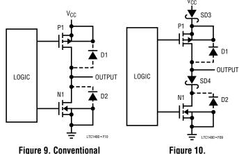
Figure 9. Conventional CMOS Output Stage
