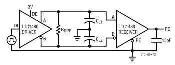
Figure 3. Driver/Receiver Timing Test Circuit
