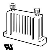
The Model 183 external multiplier enables an iron-vane type voltage meter to monitor up to 1000AC volts. An external multiplier is used with a 150AC voltmeter that is scaled proportionally to your measurement range. Simpson's AC meters having a range of 500 volts or higher are furnished with the Model 183. Simpson's external multipliers are available for immediate delivery from your local distributor. Other intermediate ranges are available on special order.
