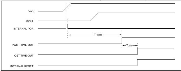
FIGURE 11-7: TIME-OUT SEQUENCE ON POWER-UP (MCLR NOT TIED TO VDD): CASE 2
