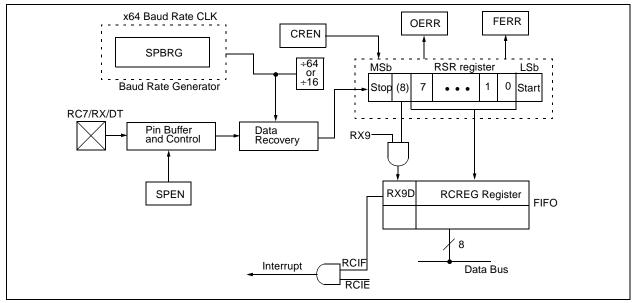
FIGURE 9-5: ASYNCHRONOUS RECEPTION
