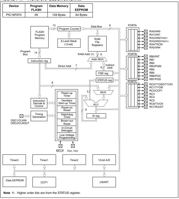
FIGURE 1-2: PIC16F871 BLOCK DIAGRAM
