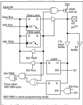
te 1: I/O pins have diode protection to VDD and Vss.
