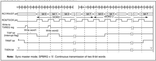
FIGURE 9-10: SYNCHRONOUS TRANSMISSION (THROUGH TXEN)
