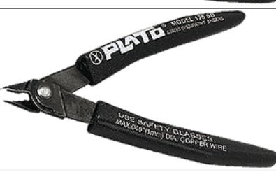
Platoshear 170 SMD - ESD Safe: Designed for use in restricted areas. The low profile cutting head width of .290" (7.38mm) and an end radius of .010" (.25mm) is designed to cut between SMD leads as close as .040"(1mm) center to center and up to .025:(0.6mm) in diameter. Includes unique SAF-T-LINK® feature for greater operator safety.
