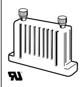
The Model 183 external multiplier enables an iron-vane type voltage meter to monitor up to 1000 AC volts. An external multiplier is used with a 150 AC voltage meter that is scaled proportionally to measurement range. Simpson's AC meters having a range of 500 volts or higher are furnished with the Model 183. Simpson's external multipliers are available for immediate delivery from your local distributor. Other intermediate ranges are available on special order.
