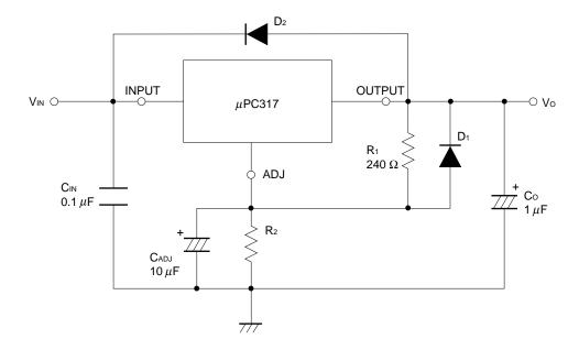
Remark R<sub>1</sub>, R<sub>2</sub>: Resistor to set the output voltage.
