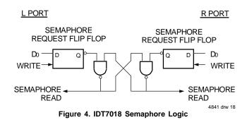
over to the other side as soon as a one is written into the first side's request latch. The second side's flag will now stay LOW until its semaphore request latch is written to a one. From this it is easy to understand that, if a semaphore is requested and the processor which requested it no longer needs the resource, the entire system can hang up until a one is written into that semaphore request latch.
