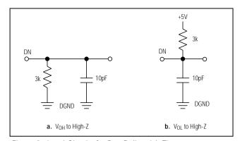
Figure 2. Load Circuits for Bus-Relinquish Time
