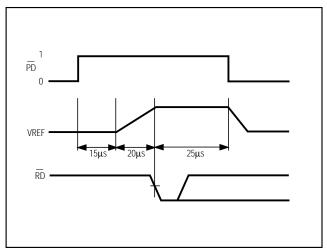
Figure 18b. Low Average-Power Mode Operation (Internal Compensation)
