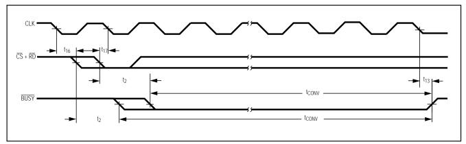
Figure 6. CS, RD, and CLK Synchronous Operation
