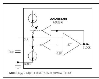
Figure 5. Internal Clock Circuit
