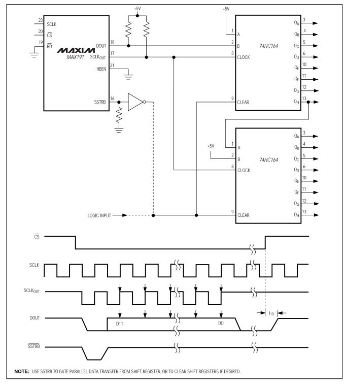
Figure 11. Simple Serial-to-Parallel Interface
