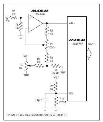
Figure 21b. Offset (±10mV) and Gain (±1%) Trim Circuit
