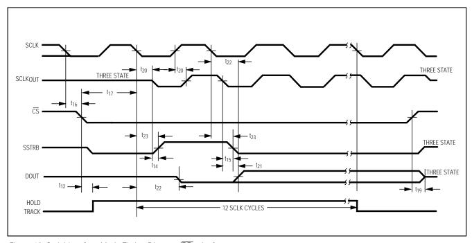
Figure 10. Serial-Interface Mode Timing Diagram ( $\overline{RD}$  = low)
