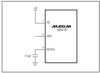
Figure 18a. Internal-Compensation Mode Circuit
