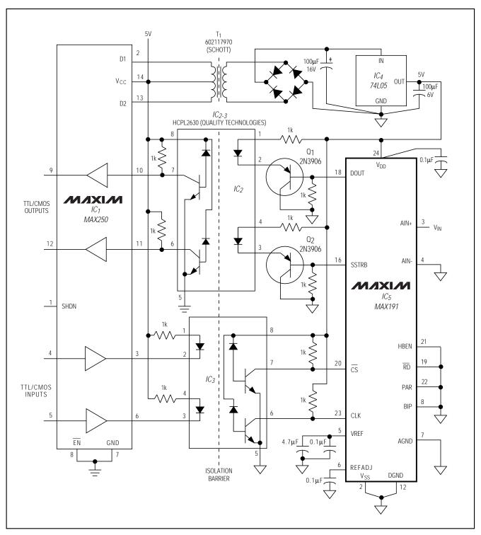
Figure 24. Isolated Data-Acquisition Circuit
