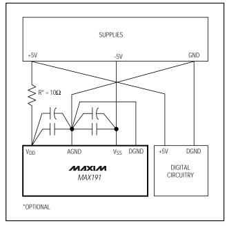
Figure 23. Power-Supply Grounding Connection
