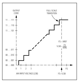
Figure 20. Unipolar Transfer Function
