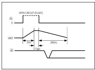
Figure 19b. Low Average-Power Mode Operation (External Compensation)
