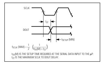
Figure 12.  $f_{SCLK}(MAX)$  is limited by the setup time required by the serial data input to the  $\mu P$ .
