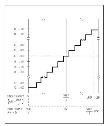
Figure 22. Bipolar Transfer Function
