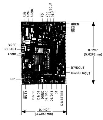
SUBSTRATE CONNECTED TO VDD
