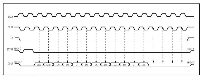
Figure 16. TMS320 Interface Timing
