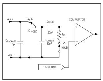
Figure 4. Equivalent Input Circuit
