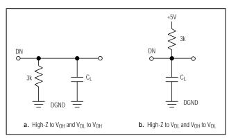
Figure 1. Load Circuits for Access Time
