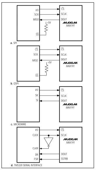
Figure 13. Common Serial-Interface Connections to the MAX191
