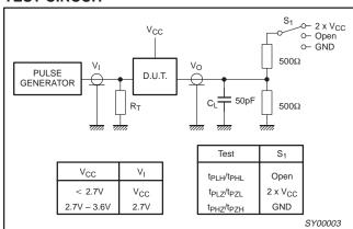
Figure 4. Load circuitry for switching times.
