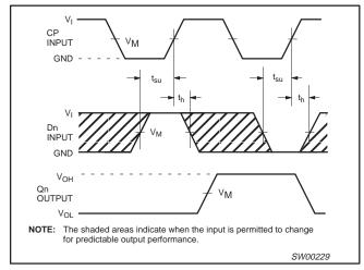
Figure 3. Data setup and hold times for the  $\mathbf{D}_{\mathbf{n}}$  input to the CP input.
