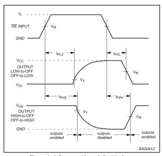
Figure 2. 3-State enable and disable times.
