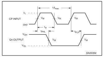
Figure 1. Clock (CP) to output  $(\mathbf{Q}_{\mathbf{n}})$  propagation delays, the clock pulse width and the maximum clock pulse frequency.
