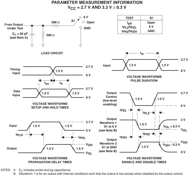
Waveform 2 is for an output with internal conditions such that the output is high except when disabled by the output control. C. All input pulses are supplied by generators having the following characteristics: PRR  $\leq$  10 MHz, Z<sub>O</sub> = 50  $\Omega$ , t<sub>r</sub>  $\leq$  2.5 ns, t<sub>f</sub>  $\leq$  2.5 ns.
