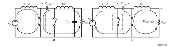
FIGURE 1. Operating Cycles of a Cuk Converter
