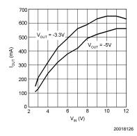
FIGURE 5. I<sub>OUT(MAX)</sub> vs V<sub>IN</sub> using 1oz. copper layout. See *Figure 14* for the test circuit.
