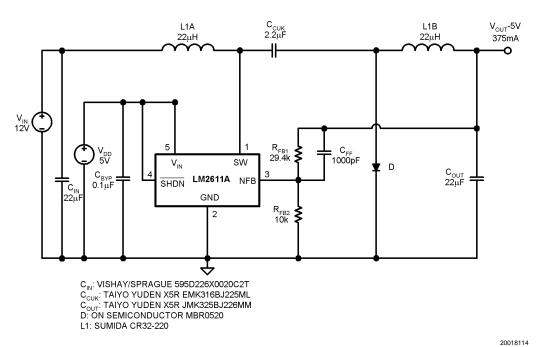
FIGURE 10. LM2611 Operating with Separate Power and Biasing Supplies
