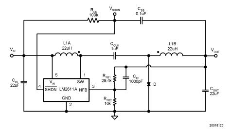
FIGURE 11. LM2611 Soft Start Circuit
