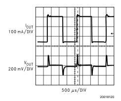
FIGURE 6. 130mA to 400mA Transient Response of the circuit in Figure 10 with C<sub>FF</sub>= 1nF
