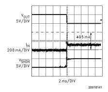
FIGURE 13. Start-Up Waveforms without Soft Start Circuit
