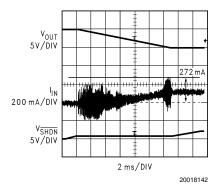
FIGURE 12. Start-Up Waveforms with Soft Start Circuit
