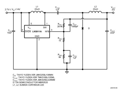
FIGURE 14. LM2611 High Current Schematic
