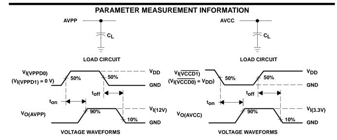
Figure 1. Test Circuits and Voltage Waveforms
