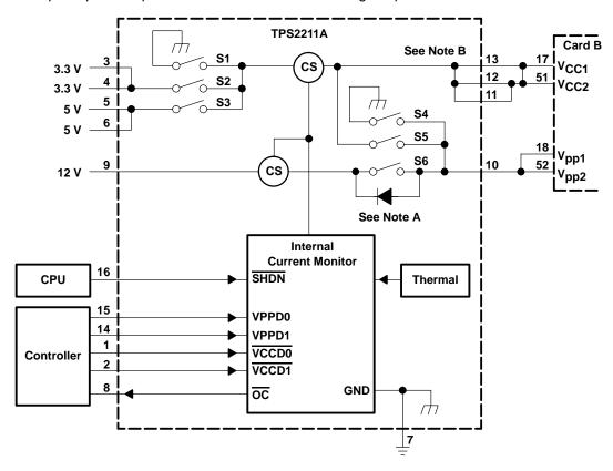
NOTE A: MOSFET switch S6 has a back-gate diode from the source to the drain. Unused switch inputs should never be grounded. NOTE B: The diagram refers to the 16-pin DB package.
