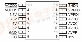
† TPS2211A is pin-for-pin compatible with TPS2211 and TPS2212.
