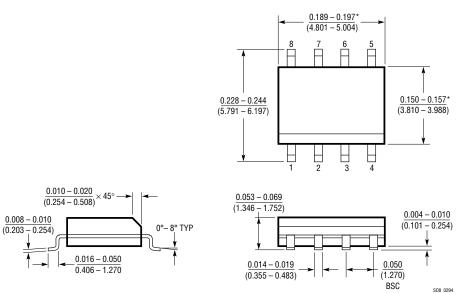
\*THESE DIMENSIONS DO NOT INCLUDE MOLD FLASH OR PROTRUSIONS. MOLD FLASH OR PROTRUSIONS SHALL NOT EXCEED 0.006 INCH (0.15mm).
