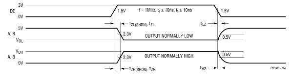
Figure 6. Driver Enable and Disable Times
