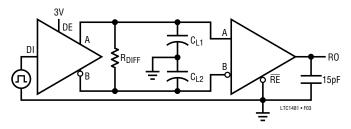
Figure 3. Driver/Receiver Timing Test Circuit
