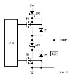
Figure 9. LTC1481 Output Stage
