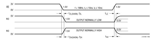
Figure 8. Receiver Enable and Disable Times
