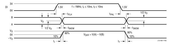
Figure 5. Driver Propagation Delays
