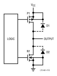
Figure 10. Conventional CMOS Output Stage
