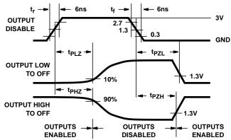
FIGURE 4. HCT THREE-STATE PROPAGATION DELAY WAVEFORM
