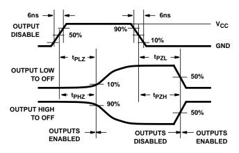
FIGURE 3. HC THREE-STATE PROPAGATION DELAY WAVEFORM
