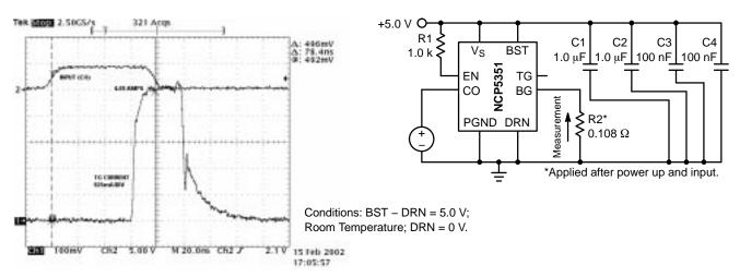
Figure 11. Top Gate Sourcing Current into 0.108  $\Omega$
