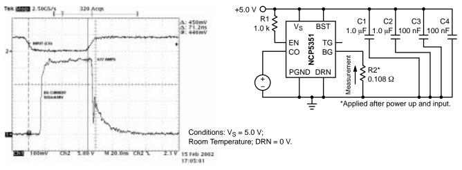
Figure 9. Bottom Gate Sourcing Current into 0.108  $\Omega$
