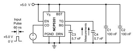
Figure 18. Bottom Gate and Top Gate Rise/Fall Time Test
