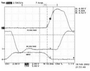
Conditions:  $V_S = 5.0 \text{ V}$ ; BST – DRN = 5.0 V;  $C_{LOAD} = 5.7 \text{ nF}$ ; Room Temperature.
