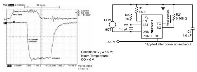
Figure 7. Bottom Gate Sinking Current from 0.108  $\Omega$
