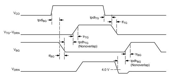
Figure 2. Timing Diagram
