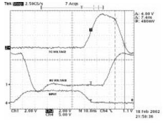
Conditions: V<sub>S</sub> = 5.0 V; BST – DRN = 5.0 V; C<sub>LOAD</sub> = 5.7 nF; Room Temperature.
