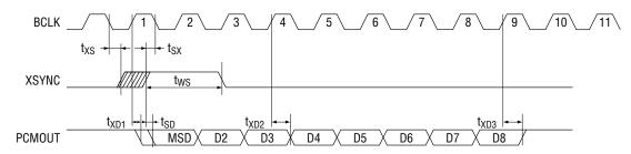
When  $t_{XS} \le 1/2$  • Fc, the Delay of the MSD bit is defined as  $t_{XD1}$ . When  $t_{SX} \le 1/2$  • Fc, the Delay of the MSD bit is defined as  $t_{SD}$ .
