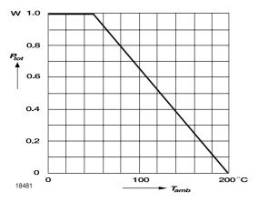
Figure 1. Admissible Power Dissipation vs. Ambient Temperature
