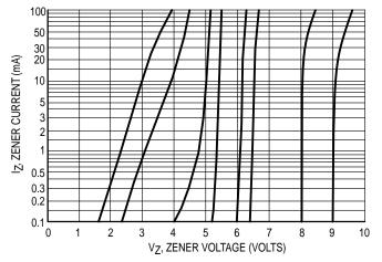
Figure 7.  $V_Z = 3.3$  thru 10 Volts
