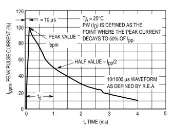
Figure 4. Pulse Waveform 10/1000
