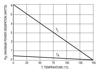
Figure 1. Steady State Power Derating
