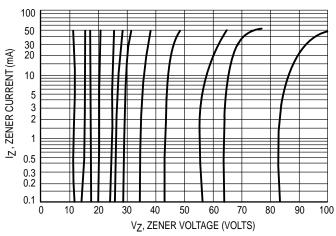
Figure 8. V<sub>Z</sub> = 12 thru 82 Volts
