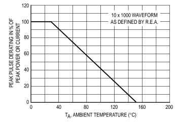
Figure 3. Pulse Derating Curve
