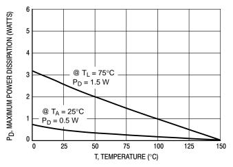
Figure 5. Steady State Power Derating
