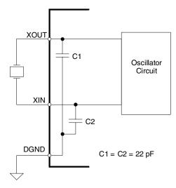
Figure 8. Oscillator Connection
